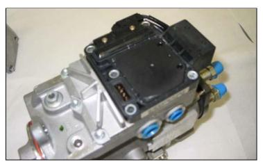
Place the plastic cover supplied in the kit on top of the pump, with the flat side up and lining up the holes for the 5 retaining screws.
