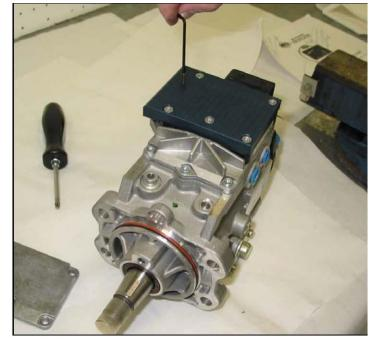
Place the piercing Allen set screw (P/N# 1502005) into the small hole on the plastic cover, and then screw it down with the supplied Allen key (P/N# 1502003) so that it is going in straight.
